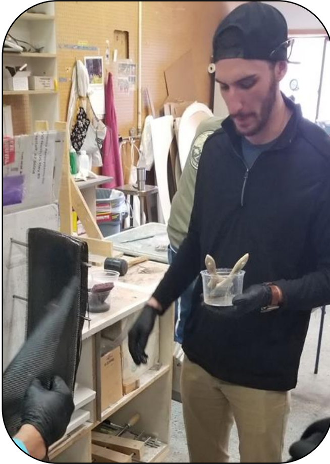
Laying up carbon fiber for wing shroud
